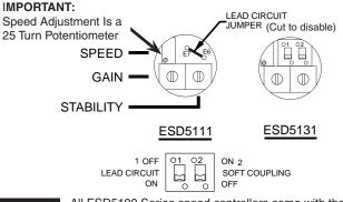
All ESD5100 Series speed controllers come with the Lead NOTE Circuit enabled. Cut the jumper between posts E6 and E7 to disable. ESD5131 has a switch to disable the Lead Circuit.
